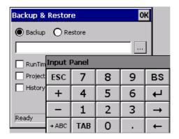
A backup copy of the components chosen through ticking can be made from here: Runtime, Project, History. It is essential to tick at least one of the components to be exported and choose a path where to save the file. The restore can be done for all exported components or through ticking, choose the component or components for which restore is to be carried out.
