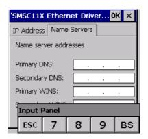
f necessary, the parameters relating to the relative DNS or AL WINS must be entered
