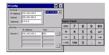
By clicking on the "IP Config" icon, the mask displaying the IP Address of the terminal and IP Address (or IP Addresses) of the devices connected via Ethernet will appear.
