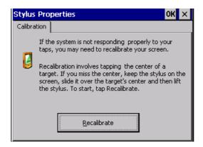
From the control panel click on the stylus icon and, subsequently, the following screens are displayed on the recalibrate key. Touch the screen near the crosses that appear on the screen.
