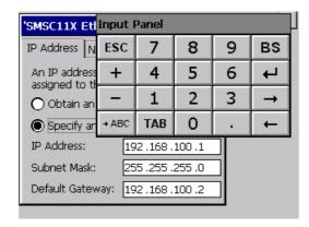
Obtain an IP address via DHCP: by selecting this option, an IP address is automatically obtained (ensure that the DHCP server is enabled on the network)
