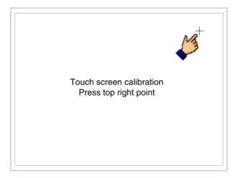
• Touch the corner indicated in the figure to complete the calibration procedure; the following page now appears
