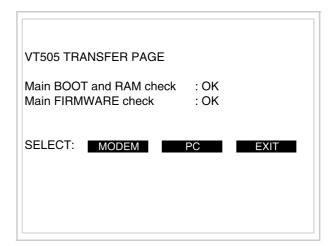
• Choose the required transfer mode: MODEM if you intend to use a modem or PC if you intend to use a serial port; touch the relevant  $\square$  on the display
