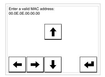
• Use the arrow 💷 to make the setting. Once the address has been confirmed the following page is displayed
