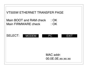
The MAC address is permanently memorized in the terminal, but should it be necessary to execute an "aided" BOOT update (see Software Manual "Chapter 14 -> BOOT update") the address is lost.
