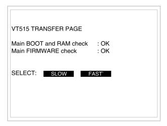
The choice should be according to the speed you intend to use for the transfer (Slow=9600bit/sec or Fast=38400bit/sec), touch the relevant  $\square$  on the display. The VT is now ready to receive (see Software Manual for the transfer).
