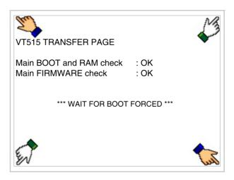
and wait a moment, or, using the appropriate button (see Page 17-24), till the VT displays the following mask
