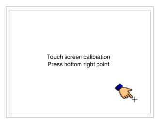
• Wait a few moments until the VT displays either the following mask or the project page (the page may be slightly different in its wording depending on which series the terminal belongs to)
