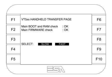
The choice should be according to the speed you intend to use for the transfer (Slow=9600bit/sec or Fast=38400bit/sec), touch the relevant  $\square$  on the display. The VT is now ready to receive (see Software Manual for the transfer).
