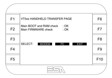
• Choose the required transfer mode: MODEM if you intend to use a modem or PC if you intend to use a serial port; touch the relevant □ on the display
