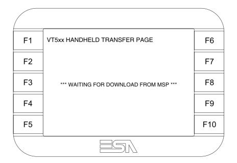
The on-screen to press depends on the port you intend to use (MSP or ASP). The VT terminal is now ready to receive (consult Software Manual for information on the transmission procedure).
