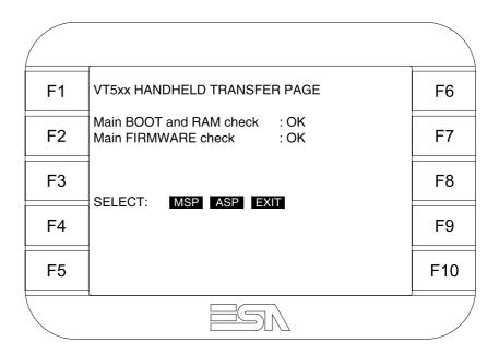
• Choose the port you intend to use for the transfer (MSP or ASP); touch the relevant  $\square$  on the display. The VT is now ready to receive (refer to Software Manual for transfer procedure).
