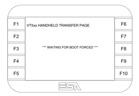
• To access the calibration page, touch the message \*\*\*WAITING FOR BOOT FORCED\*\*\* three to six times in quick succession
