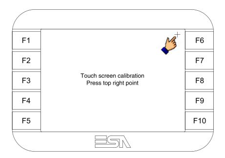
• Touch the corner indicated in the figure to complete the calibration procedure; the following page now appears
