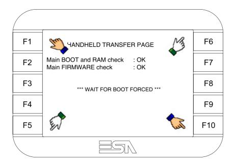
and wait a moment, or, using the appropriate button (see Page 19-21), till the VT displays the following mask
