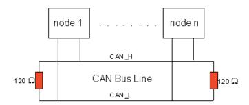
CAN is a 2-wire bus system in which all participants are connected in parallel (that is to say with short stub lines). The bus must be terminated at both ends with a 120 (or 121) ohm terminating resistor in order to prevent reflections. This is necessary even in case of very short line lengths!
