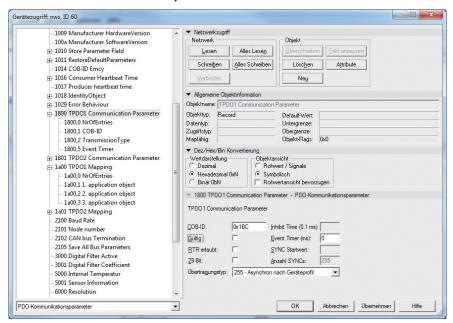
2. The mapping entries of TPDO 1 are modified in object 1A00A, and then the number of the actual entries is updated in 1A00 00h:
