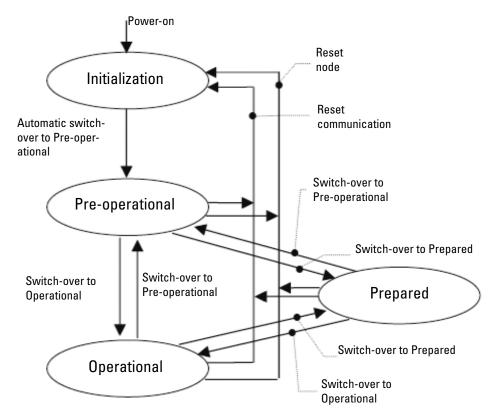
**Initialization:** this is the initial state after the power supply is applied, following a device Reset or Power ON. After performing the reset/initialization routines, the node switches automatically to the Pre-operational status. The LEDs display the momentary status.
