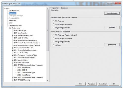
Switch then over to Operational Mode. The mapped objects of TPD01 are sent in a 100ms cycle:
