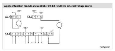
Minimum wiring required for operation
