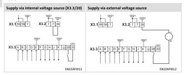
Minimum wiring required for operation
