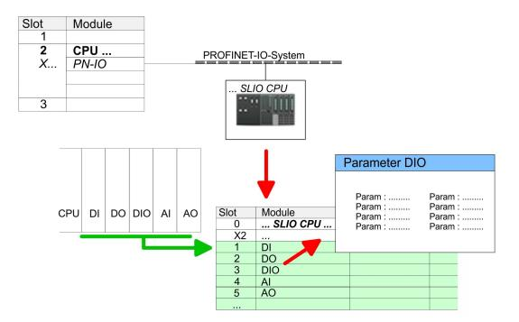
**Parametrization** For parametrization double-click during the project engineering at the slot overview on the module you want to parametrize. In the appearing dialog window you may set the wanted parameters.
