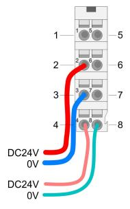
For wires with a core cross-section of 0.08mm<sup>2</sup> up to 1.5mm<sup>2</sup>.
