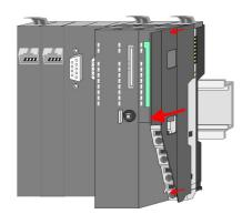
**1.** Before mounting the periphery modules you have to remove the bus cover at the right side of the CPU by pulling it forward. Keep the cover for later mounting.
