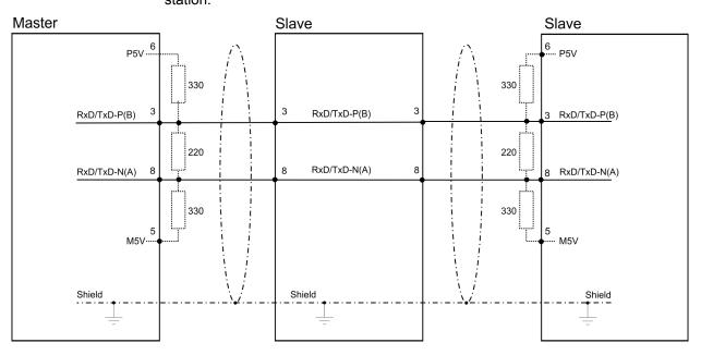
The PROFIBUS line has to be terminated with its ripple resistor. Please make sure to terminate the last participants on the bus at both ends by activating the terminating resistor.
