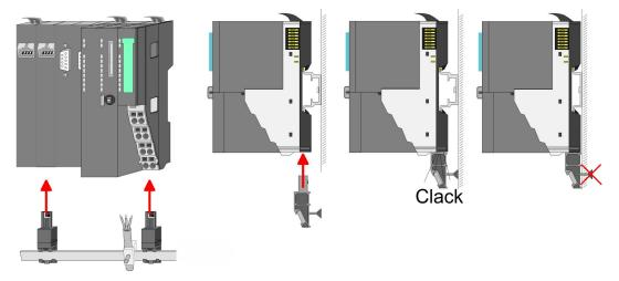
**3.** Attach the cables with the accordingly stripped cable screen and fix it by the shield clamp with the shield bus.
