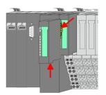
For demounting and exchange of a (head) module or a group of modules, due to mounting reasons you always have to remove the electronic module <u>right</u> beside. After mounting it may be plugged again.
