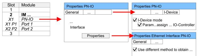
Create an I-Device GSD file and install it at your hardware catalog with 'Options → Create GSD file for I-Device'. Open the hardware configuration of your higher-lever VIPA CPU and connect your Siemens I-Device from 'Preconfigured Stations'.
