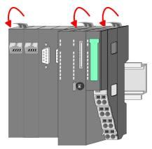
**2.** Turn the locking lever upwards, place the CPU at the mounting rail and turn the lever downward.
