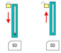
To remove, slide the sliding mechanism up again and push the storage media against the spring pressure until it is unlocked with a click.
