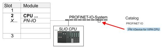
Use as I-Device > Configuration in the Siemens SIMATIC Manager
