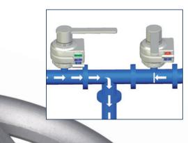
Now the operator inserts the key  ${\bf B}$  (blue) into the left interlock. The lock is released and the operator can open the left valve. As soon as the valve is open, the key  ${\bf C}$  (green) can be removed. Now the media can flow in the left pipe. By removing the key, this valve is also locked and can no longer be operated.
