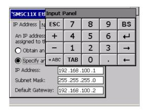
Obtain an IP address via DHCP: by selecting this option, an IP address is automatically obtained (ensure that the DHCP server is enabled on the network)
