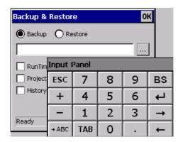
A backup copy of the components chosen through ticking can be made from here: Runtime, Project, History. It is essential to tick at least one of the components to be exported and choose a path where to save the file.
