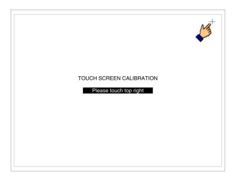
• Touch the corner indicated in the figure to complete the Calibrazione procedure; the following page now appears
