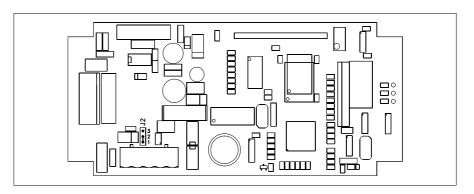
The device in question integrates the termination resistances of the serial line (typically 120 ohms) which can be inserted by means of a jumper (preset on 1-2, line not terminated). To activate the termination:
