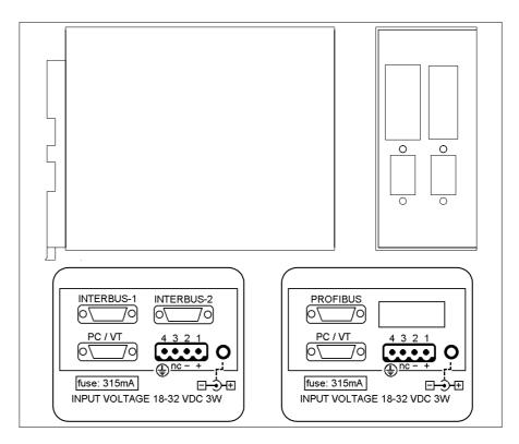
The casing is the same both for the Interbus-S and the Profibus-DP networks; a label is attached to indicate which network is contained.
