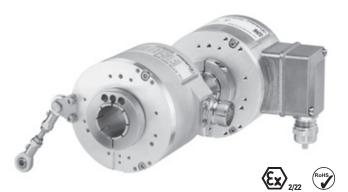
The Sendix Heavy Duty H120 were especially developed for large motors and generators. They are highly accurate and extremely robust thanks to HD-Safety-Lock™ – the Heavy Duty hollow shaft design of the latest generation with sturdy bearing construction and integrated bearing isolation. The dual protection of the shaft, the wide temperature range and the high protection level allow for use even under the harshest conditions.
