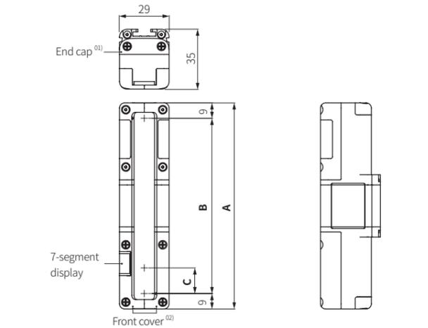
01) When removing the end cap, there is the lamp output terminal (top) or the power supply terminal (bottom).
