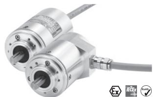
The Sendix 7063 absolute multiturn encoders offer Ex protection in a compact 70 mm seawater resistant housing, with an SSI or BiSS-C interface and optical sensor technology.
