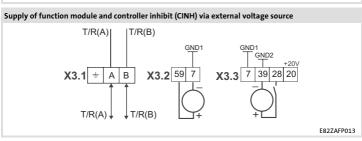
Minimum wiring required for operation
